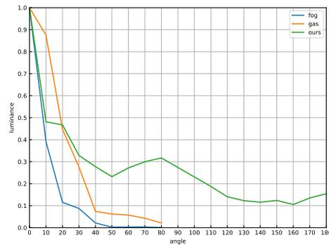
**Fig. 5.** Decrease of the luminance value with respect to the angle. The maximum value is 1 and the ratio is as shown. Glass beads possess a wide viewing angle, whereas fog and gas possess a large brightness value (depending on the viewing angle).
