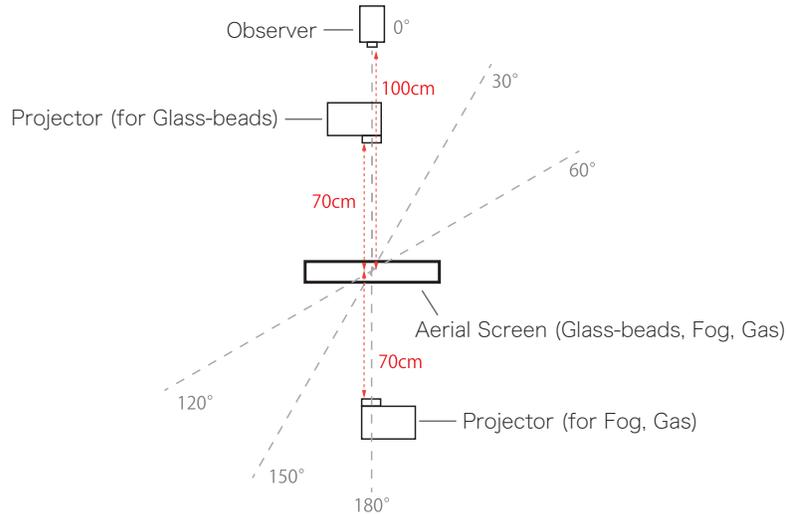
**Fig. 2.** Configuration of experimental setup. The observer represents people, cameras, and luminance meters. The same configuration was used in all the experiments. Note that the position of the projector varies but the distance from the screen remains the same.
