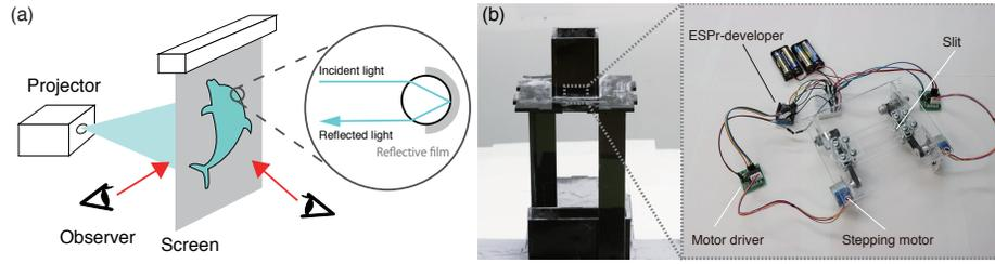
**Fig. 1.** The retroreflective particles fall from the control device. By projecting images from the projector on the screen, observers can clearly see the aerial images from all directions. (a) System overview. (b) Prototype and control device.
