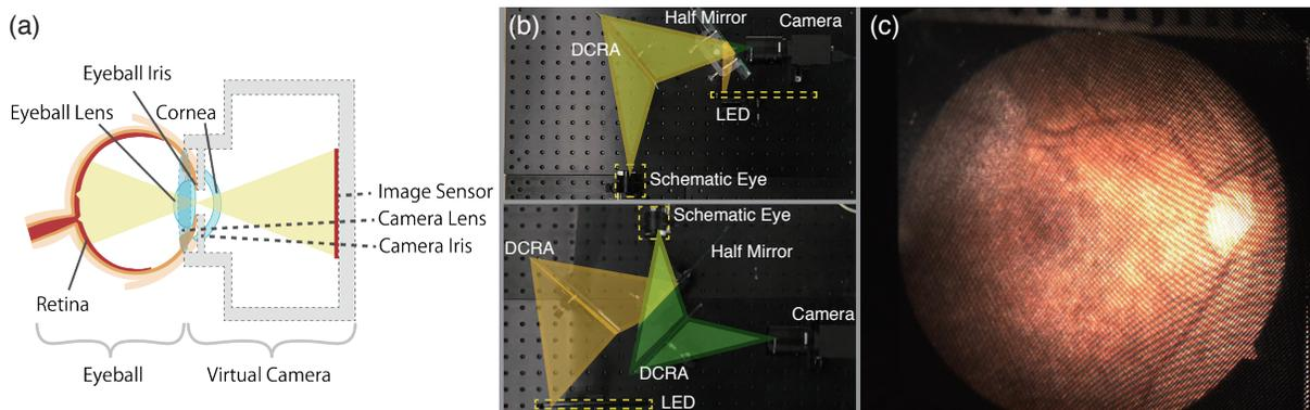
**Figure 1: (a) Concept of virtual camera that overlaid to the eyeball using DCRA. (b) Our optical system consisted of camera and two DCRA and light source. (c) A captured image. We used the schematic eye instead of the real eye.**
